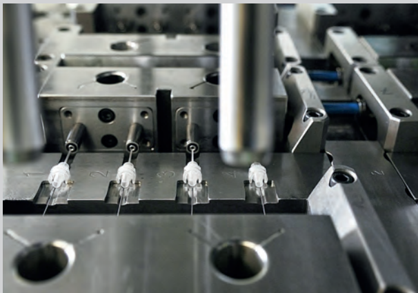
Part "venting adapter" in the moving mould half with slide units (above). Valve gate hotrunner system with slim nozzles and compact manifold for production of the venting adapter (right).
