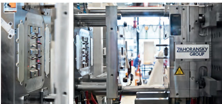
Mould with lifting contour plate and cores with stripper plate on hotrunner side (left). Laser scanning is used to check whether each cavity is fed when inserting the needles (far left).
